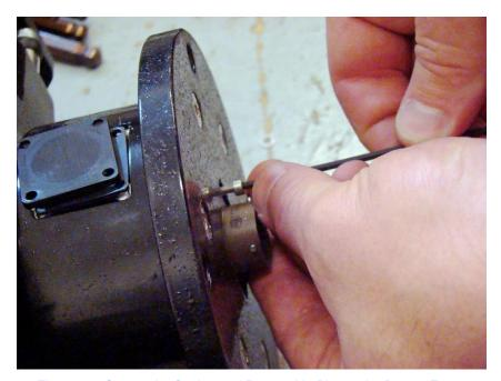
Figure 2-9 Secure the Gasket and Removable Plug to the Bottom Egress
