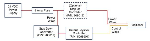
Figure 2-12 Powered with 24 VDC
