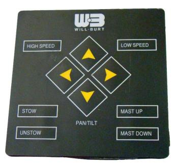
Figure 6-2 Panel Mount Controller (P/N: 4270601)
