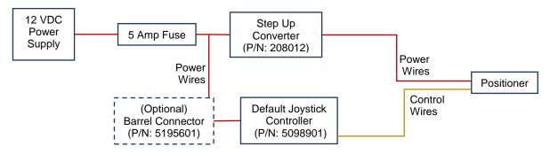
Figure 2-11 Powered with 12 VDC
