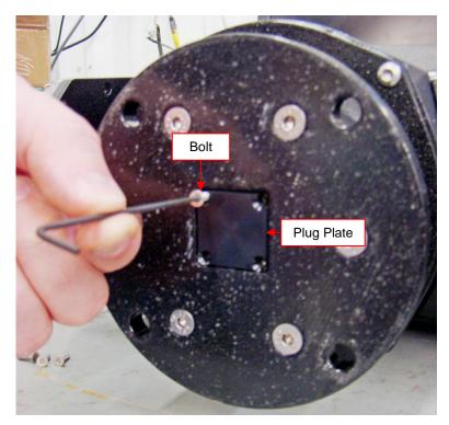
Figure 2-6 Remove the (4) Bolts Securing the Plug Plate
