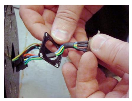
Figure 2-8 Pull the Wires out the Bottom of the Positioner
