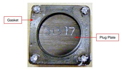
Figure 2-7 Remove Plug Plate and Gasket
