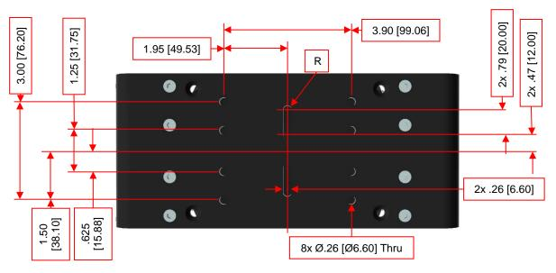
Figure 2-14 Payload Mounting Hole Pattern
