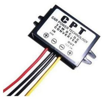
Figure 1-8 Step Down Converter
