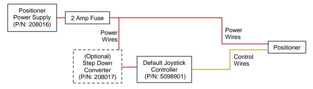
Figure 2-13 Powered with VAC
