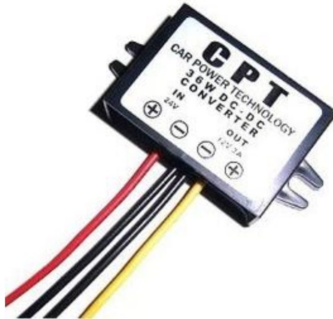
Figure 1-8 Step Down Converter
