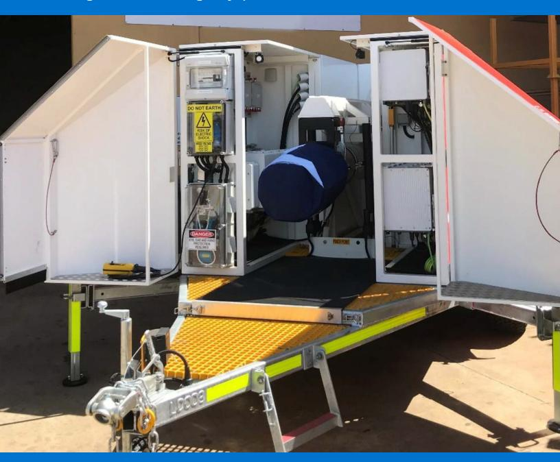
The mast is integrated onto a tilting system at ground level negating the need for any work from a ladder or platform.
