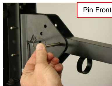
Figure 4-49 Pick an Angle for the Extension Arm and Pin into Place
