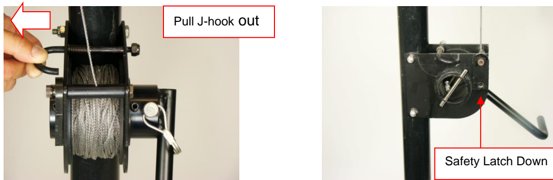
Figure 4-81 Unlock Winch Spool
