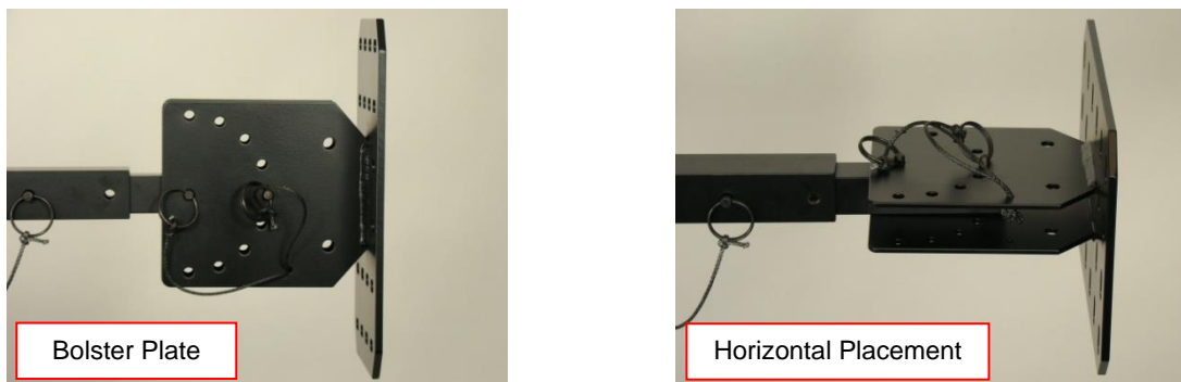
Figure 4-53 Connect the Bolster Plate to the Carriage
