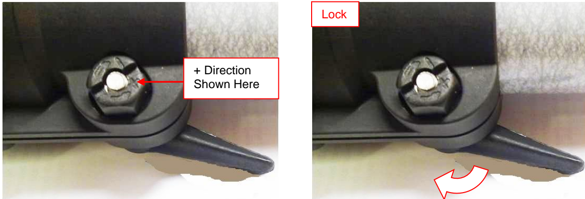
Figure 7-4 Turn the Nut by Hand in the “+” Direction Shown on the Nut to Ensure the Clamp is Tight
