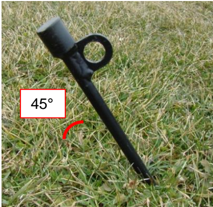
Figure 4-30 Drive Each Stake into the Ground at a 45° Angle
