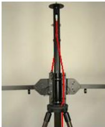
Figure 4-69 Cable Path Shown in Red
