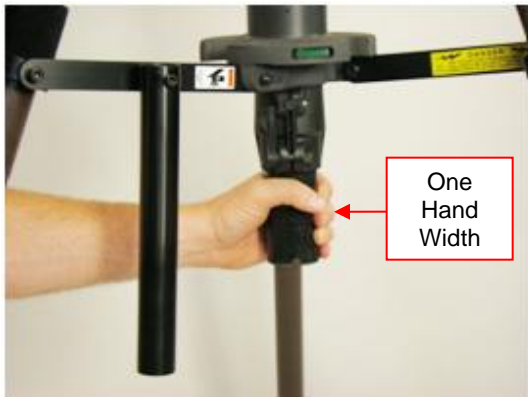
Figure 4-40 Lower Top Tube until There is One Hand Width from the Bottom of the Tube and Lock the Lower Clamp
