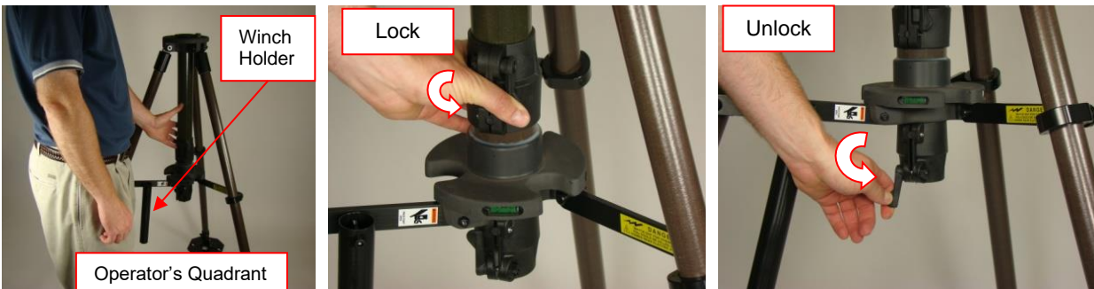
Figure 4-13 Lock the Upper Clamp and Unlock the Lower Clamp
