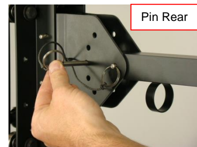
Figure 4-49 Pick an Angle for the Extension Arm and Pin into Place
