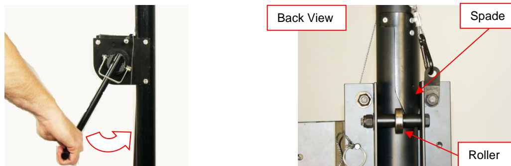
Figure 4-82 Turn the Winch Handle Counterclockwise to Raise the Payload
