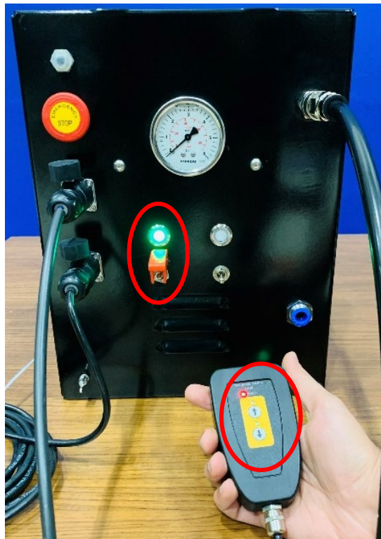
Figure 3-6 HHRC is Powered On
