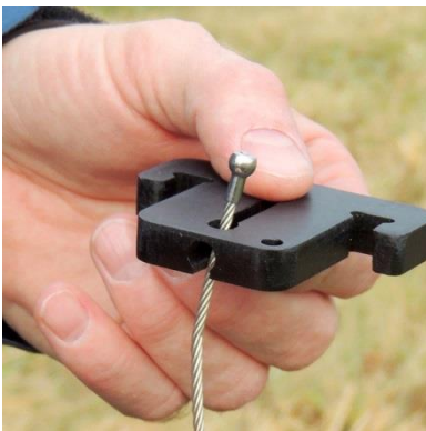
Figure 4-28 Put Ball End of Cable Through the Bottom Hole
