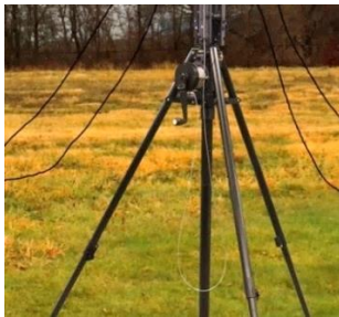
Figure 4-56 Leave Cable Loose While Deploying the Mast
