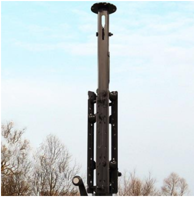
Figure 4-43 Slide EZ RAZE Top Tube Down the Carriage
