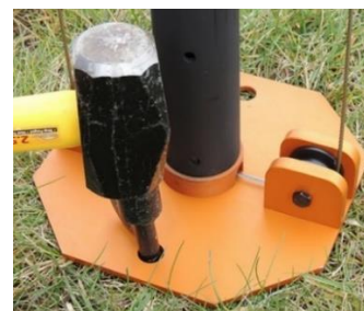
Figure 4-61 Use Hammer to Drive in Stake
