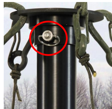
Figure 4-11 Loosen the Pin of the 4-Way Guy Collar
