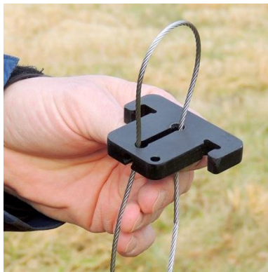
Figure 4-29 Thread the Cable End Back Through the Top Hole
