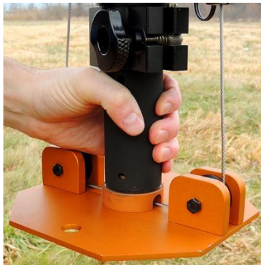
Figure 4-34 One Hand Width Below the Clamp
