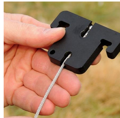
Figure 4-30 Pull the Slack Out From the Bottom of the Key
