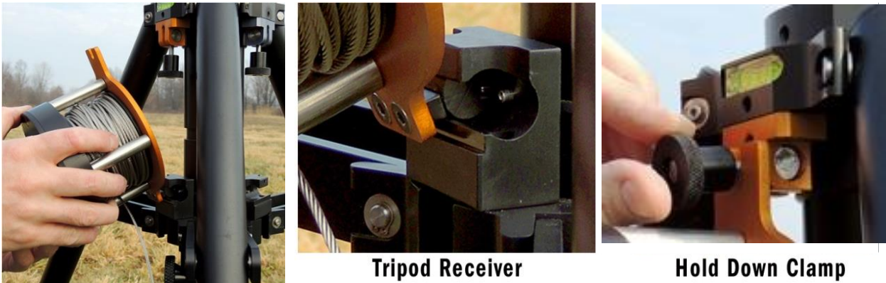
Figure 4-24 Insert Orange Barrel of the Orange Winch into the Tripod Receiver
