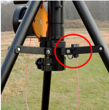
Figure 4-31 Place the Key Between the Leg Braces Opposite of the Orange Winch
