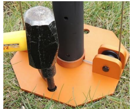
Figure 4-38 Use Hammer to Drive in Stake
