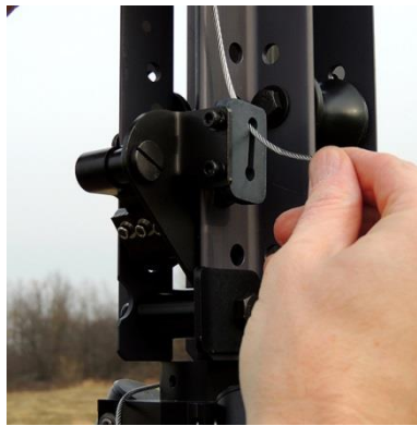
Figure 4-52 Seat Ball End of the Cable into the Recess in the Bottom of the Receiver Plate
