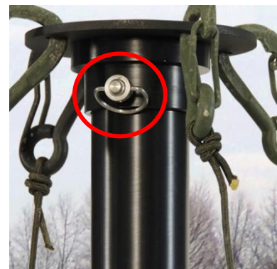
Figure 4-22 Loosen the Pin of the 4-Way Guy Collar
