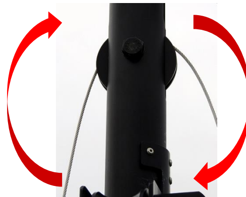
Figure 4-50 Feed the Cable Through the Top of the Top Pulley and Back Down the Other Side of the Carriage
