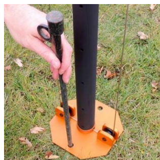
Figure 4-60 Stake the Base Plate
