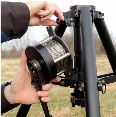
Figure 4-46 Insert the Round Key of the Blue Winch into the Tripod Receiver
