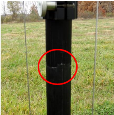
Figure 4-33 Ensure Locking Tabs Fully Engage
