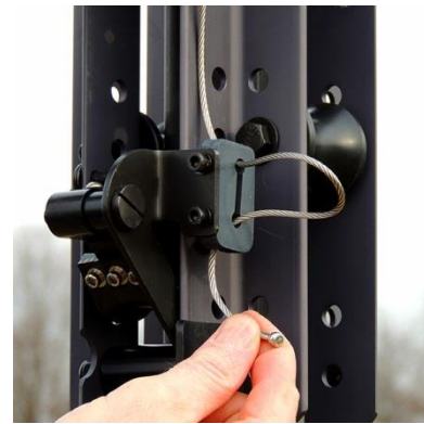
Figure 4-53 Feed End of Cable Through the Bottom Hole in the Receiver Plate
