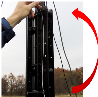
Figure 4-49 Feed Cable Through the 2 Eyelets on the EZ RAZE Carriage
